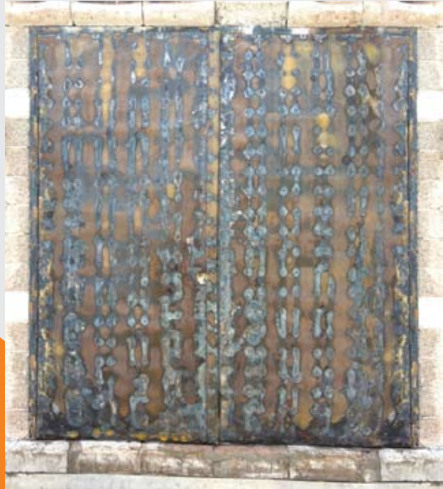
Post Test photo after UL 10C Positive Pressure (3 Hours)
